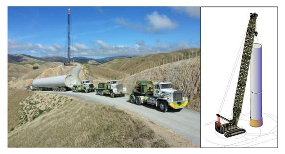
Figure 16 Example of Tower Section Delivery from a Historic Project
