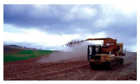
Figure 10 Straw Mulching to be Used in Conjunction with Surface Roughening.
